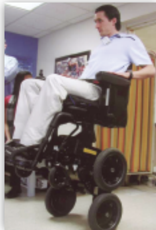
The iBOT mobility system available at Kessler lets patients climb stairs, reach high shelves and negotiate rough terrain.
